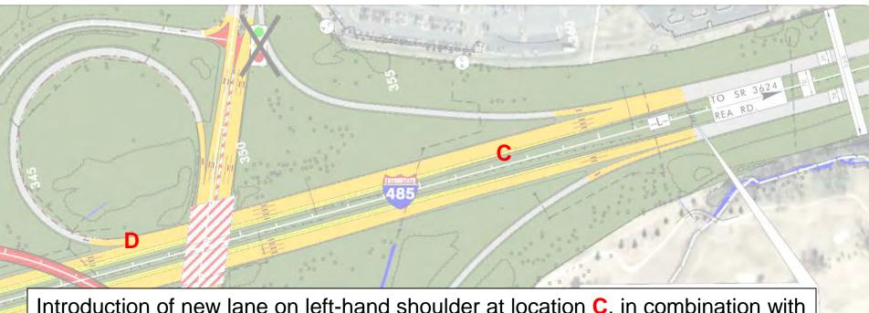
Introduction of new lane on left-hand shoulder at location **C**, in combination with loss of right-hand lane at location **D**, will cause many drivers to shift one lane to the left.
