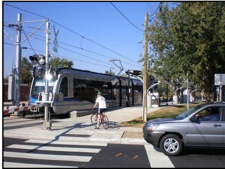
At-grade configuration example.
