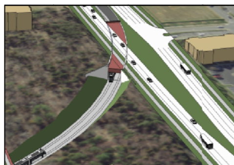
Underpass configuration example.
